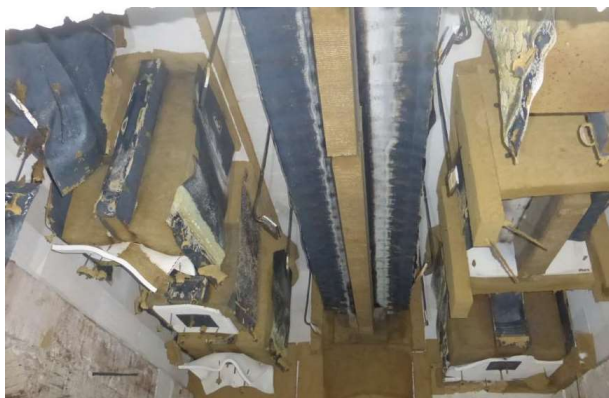
a) Disbonding of the fire-exposed steel sheets of sandwich panels
