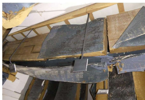
b) Falling down of protection from the bottom flange of the loaded beam
